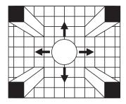
The view distance ratio is about 1 foot of viewing distance to each inch of the diameter of the dome. Due to the nature of these domes, they are made in only an 18" and 22" model. These domes are also available in See-Through mirror and transparent colors for surveillance cameras.
